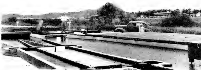
2. Tide-control structures simulated in the half-mile-long hydraulic model of a sea-level canal built to the alignment of the existing canal. To the left is the tide lock. The man is standing over the navigable pass gate, and to his left is the water-control structure. During tests the model is covered with canvas, as at the right, to shield it from the wind.
